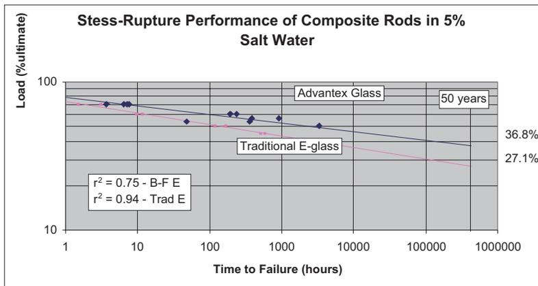
Long-term durability in demanding operating conditions is one of the key features that defines the value of composite materials. To improve the understanding of long-term performance and provide a basis for structural design, stress-rupture tests were conducted on 0.25-inch (6.4-mm) diameter pultruded rods. Exposing the test coupons
