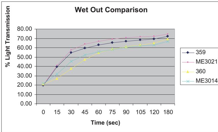
The above graph was generated using an internal Owens Corning customer mimic. This test is strictly comparative, and shows relative wet out differences between products. All products shown are Owens Corning products, and the information is to aid in finding the best product for the customer's process. Test equipment specified under ASTM
